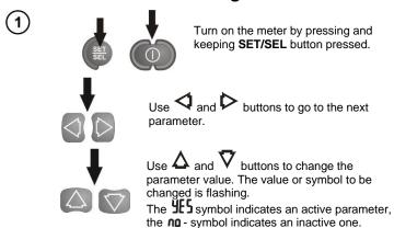
2 Set the parameters according to the following algorithm:
