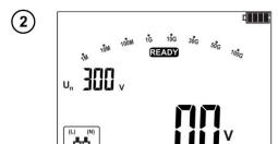
After inserting WS-04 / WS-11 into the socket, the screen displays a message indicating the detection of the adapter.
