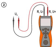
Connect the meter to a voltage source.
