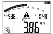
The meter measures the insulation resistance for selected pairs of leads in the following order: L-N, L-PE, N-PE.
