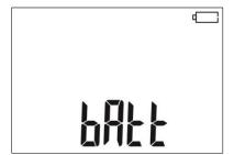
Batteries / rechargeable batteries fully discharged.
